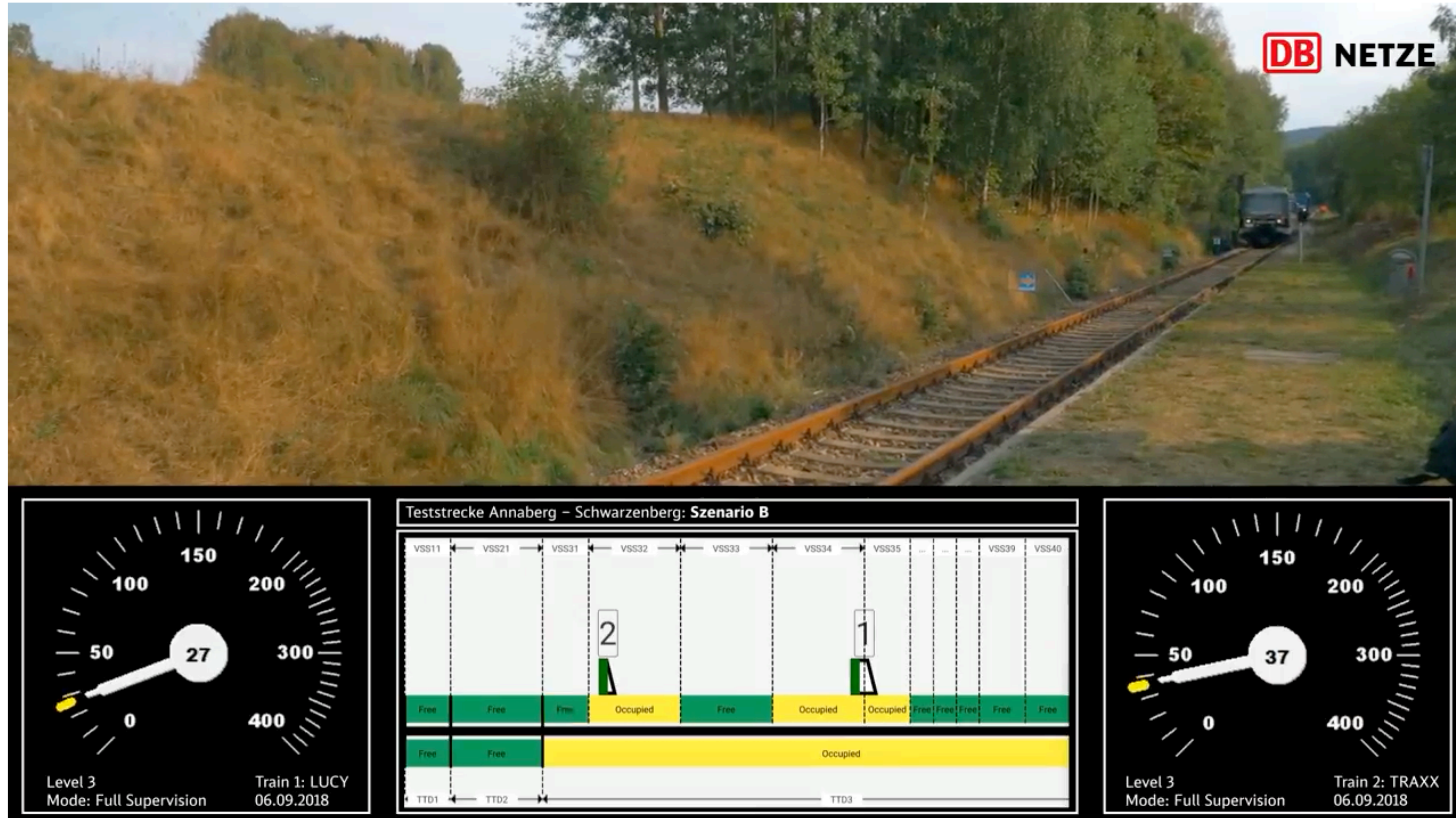
Train 2 following Train 1 (Lucy) on the same occupied track section, but on different virtual subsections
